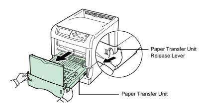
2 Wipe away the paper dust on the registration roller and the paper ramp using the wiper cloth included in the toner kit.
